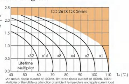
$I_A$ = actual ripple current at 100kHz.  $I_R$ = rated ripple current at 100kHz. 105°C
